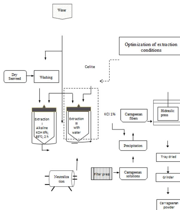
Figure 1. Extraction process of carrageenan on pilot plant scale
