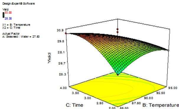
Figure 2. 3D graphic surface optimization of carrageenan yield versus extraction temperature and extraction time
