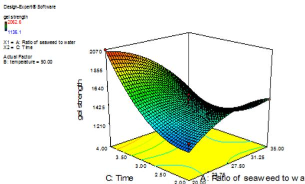
Figure 3. 3D graphic surface optimization of carrageenan gel strength versus ratio of seaweed to water and extraction time
